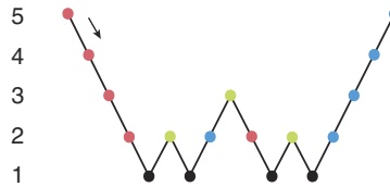
Figure 6. Schematic representation of the W^3/V(v_1, v_2) cycle on a grid with 5 levels. At red, blue, green dots v_1, v_2, v_1 + v_2 SIMPLE relaxations are performed, respectively. At black dots either direct solution or many relaxations are performed.
